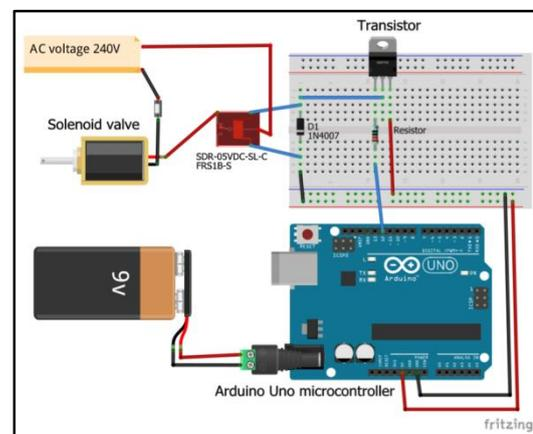
Figure 2 The Arduino controller circuit system.
