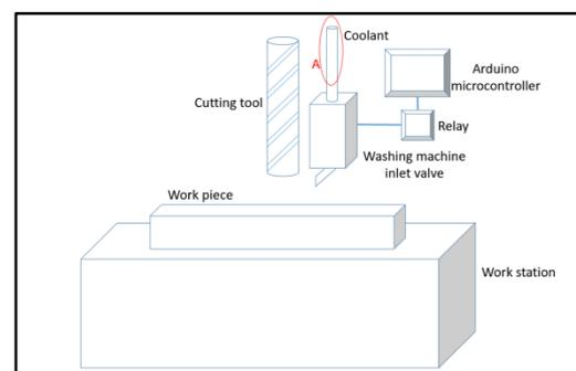
Figure 1 The overall concept of the automated coolant supply system.
