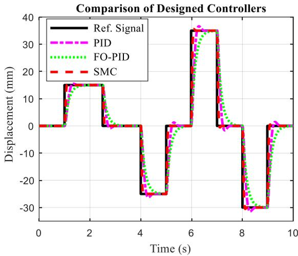
Figure 1 The performance produced by each controller.
