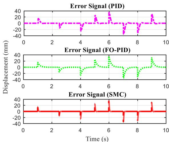
Figure 2 The error signals for PID, FOPID, and SMC.
