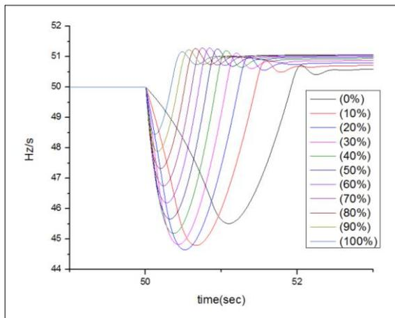
Figure 3: Frequency signal during islanding (deficit power mismatch).
