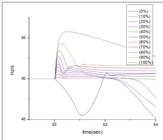
Figure 2: Frequency signal during islanding (surplus power mismatch).
