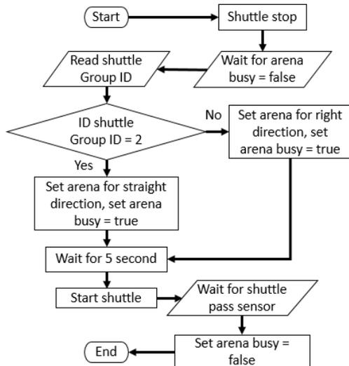
Figure 3 Structure of control logic at station 1
