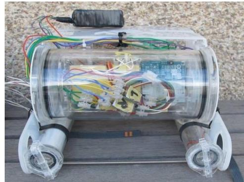
Figure 2 UTeM Panther-J AUV based on OpenROV platform.
