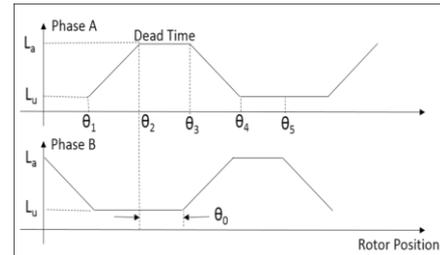
Figure 2 Typical overlapping inductance profile [1]
