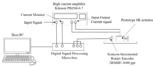
Figure 3 Measurement setup
