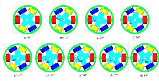
Figure 4 Initial position of the rotor from 0° to 80° with interval of 10°
