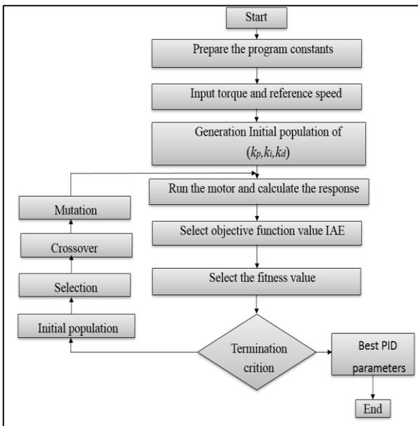
Figure 3. Flow chart for Genetic Algorithm tuning PID.
