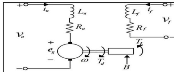
Figure 1. Equivalent circuit of the DC motor.
