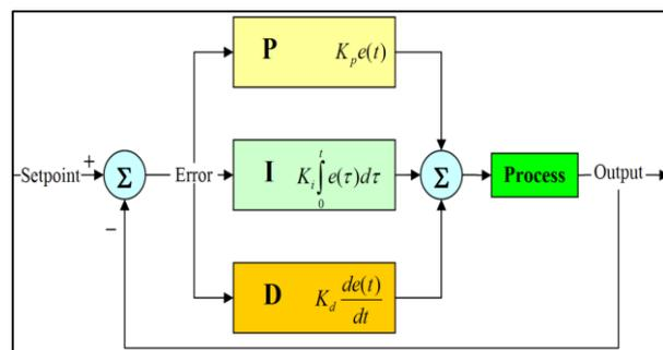
Figure 2. Equivalent circuit of PID controller.
