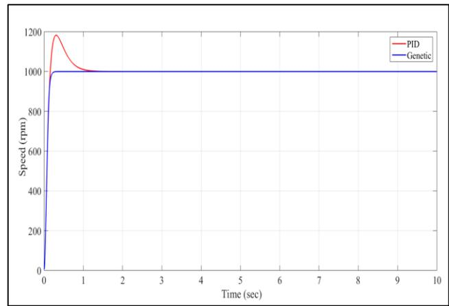
Figure 4. PID and Genetic Algorithm controller responses.
