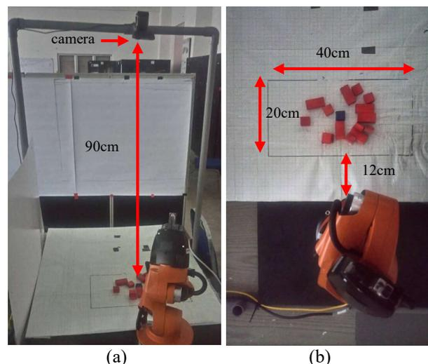
Figure 1: Full experimental setup: Kuka Youbot Robotic arm mounted on a platform with a camera overlooking the designated workspace and the pseudo duplo bricks. The task is to remove the noise objects (red) leaving only the object of interest (blue) in the works. (a) experimental
