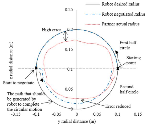
Figure 2 Trajectory of robot in negotiation of circular motion.
