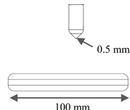
Figure 1 R0.5-Plane electrode configuration.
