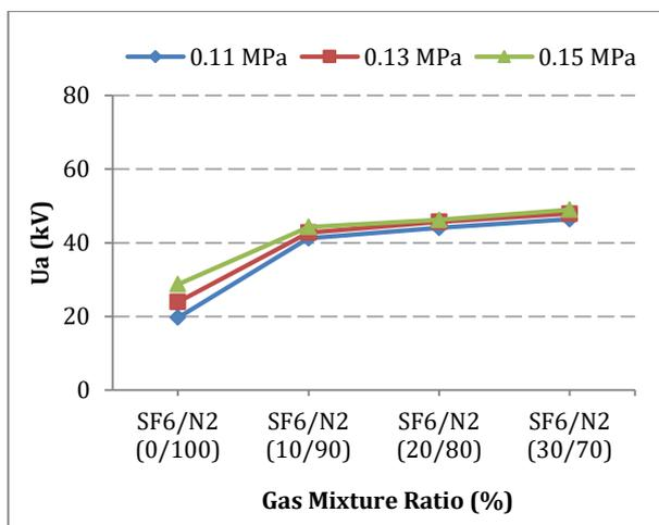
Figure 3 Mean AC breakdown voltages of SF<sub>6</sub>/N<sub>2</sub> gas mixtures at 30 mm gap distance.
