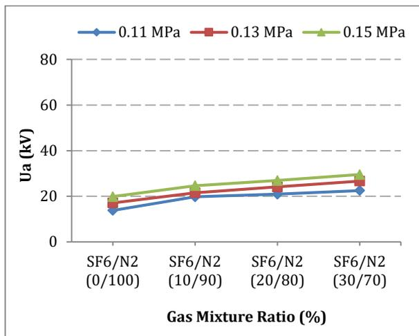
Figure 2 Mean AC breakdown voltages of SF<sub>6</sub>/N<sub>2</sub> gas mixtures at 10 mm gap distance.
