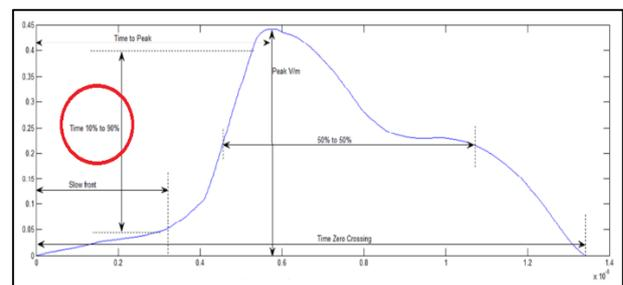
Figure 1: 10% to 90% Fast Transition (Adapted from S.N.M Arshad, (2014)).
