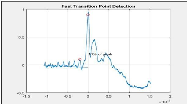
Figure 3: False Fast Transition Detection with 250 samples time of interval (The first red dotted lies outside the first return stroke).
