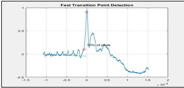
Figure 2: Accurate Fast Transition Detection with 210 samples time of interval (Both red dotted lie in the first return stroke).
