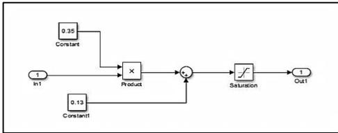
Figure 4: Linear control surface approximation method.
