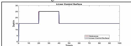
Figure 6: System response for linear control surface approximation.
