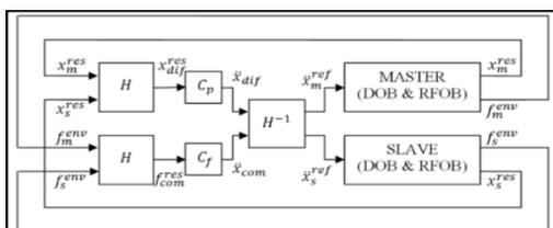
Figure 1 Block diagram for bilateral control system
