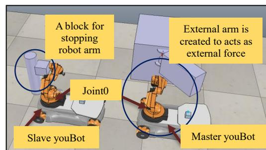
Figure 2 Overall view for bilateral control master-slave youBot system
