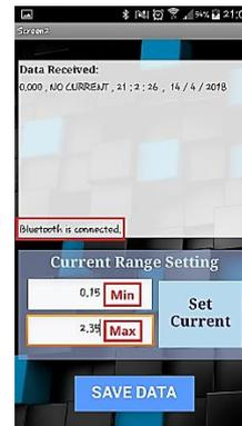
Figure 3 Android App for communication with the digital ammeter
