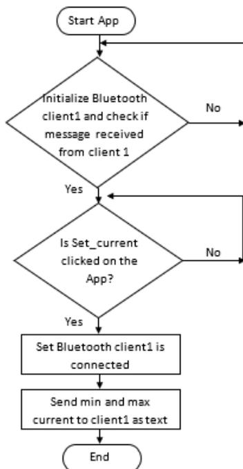
Figure 2 The flow diagram for the App design.
