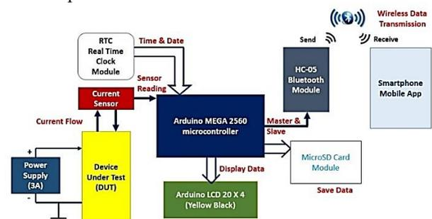
Figure 1 Digital Ammeter System Block Diagram with Bluetooth Communication.
