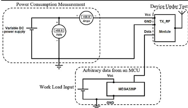
Figure 2 Evaluation experiment set-up.
