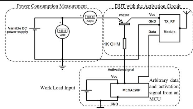
Figure 3 Proposed switching circuit.
