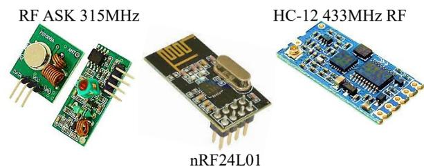
Figure 1 Wireless modules used in this research.
