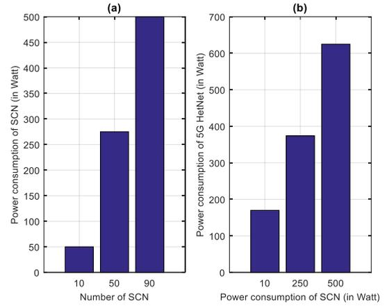
Figure 2 (a) Power consumption performance for three different traffic loads (b) 5G HetNet power consumption for three different traffic loads.
