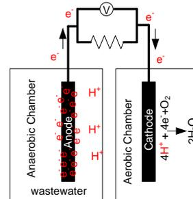
Figure 2 Double Chamber MFC.
