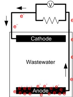
Figure 1 Single Chamber MFC.
