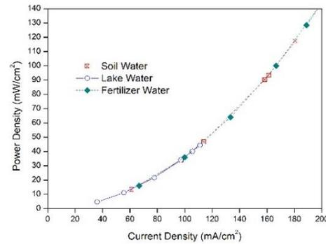
Figure 4 Performance of waste water test for double chamber MFC
