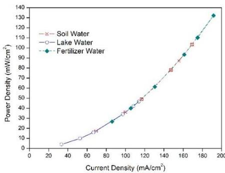
Figure 3 Performance of waste water test for single chamber MFC.
