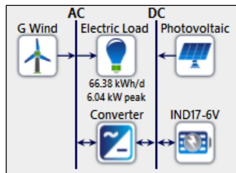
Figure 1: Schematic diagram of hybrid system.
