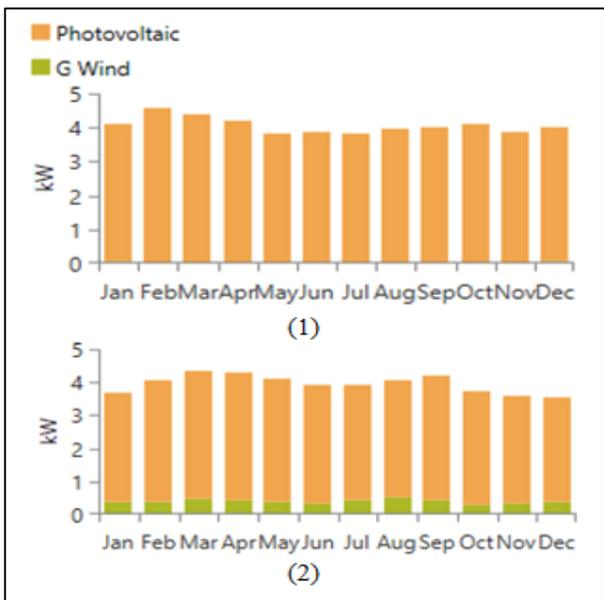
Figure 3: Monthly power penetration of Photovoltaic/wind (1) Kampung LB Johnson, Malaysia; (2) Adrar city, Algeria.
