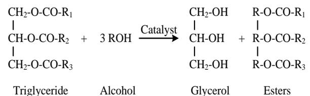
Figure 1: Molecular representation of a transesterification reaction.
