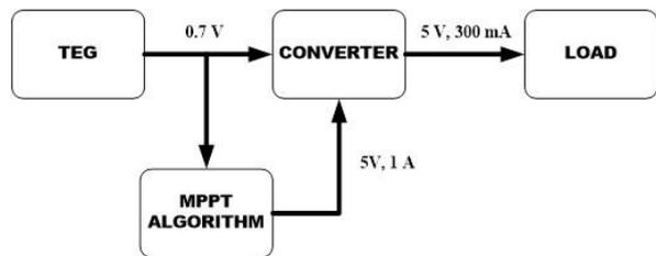
Figure 1 Block diagram for TEG system proposed
