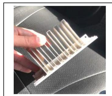
Figure 2 Custom-made heatsink.
