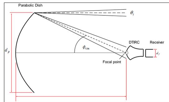
Figure 1 Illustration of PD concentrator with secondary concentrator.
