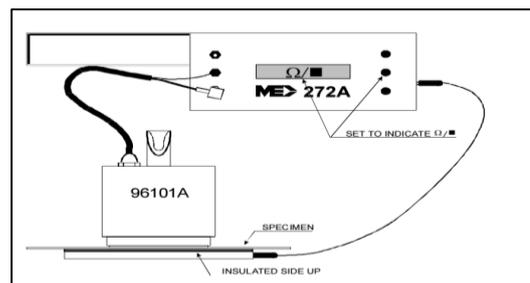
Figure 1 Portable resistivity meter set up
