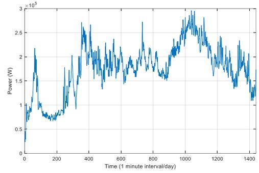
Figure 3 The aggregated load profile
