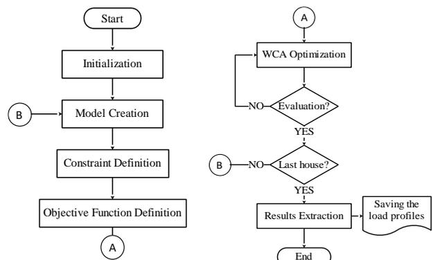
Figure 1 Stochastically load profile generation using WCA
