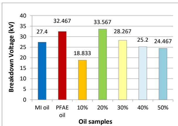
Figure 2 Average breakdown voltage ester contents.
