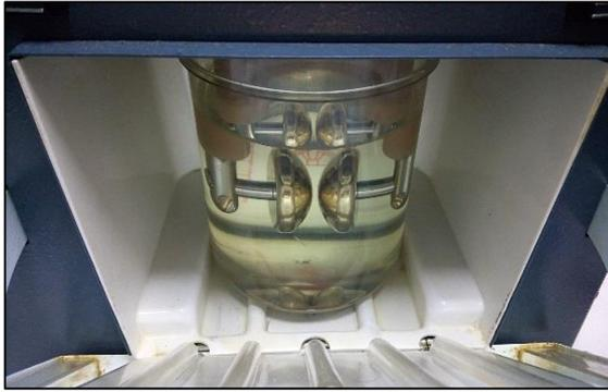
Figure 1 Electrode configuration for breakdown test.
