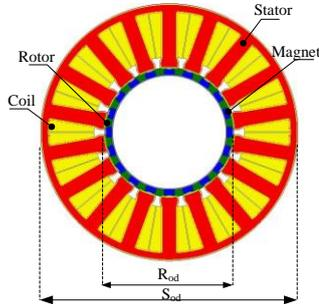
Figure 4 Hollow rotor basic structure.
