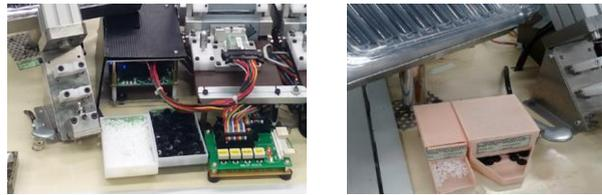
Figure 6 Old layout of parts container and new layout of parts container for Assembly station process number 5.
