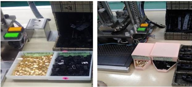
Figure 4 Old layout of parts container and new layout of parts container for Assembly station process number 3.
