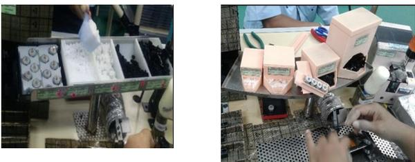
Figure 5 Old layout of parts container and new layout of parts container for Assembly station process number 4.
