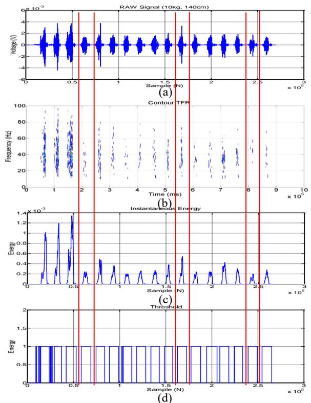
Figure 2 task of lifting: (a) raw signal of manual lifting task, (b) spectrogram representation, (c) instantaneous energy, (d) threshold calculation
